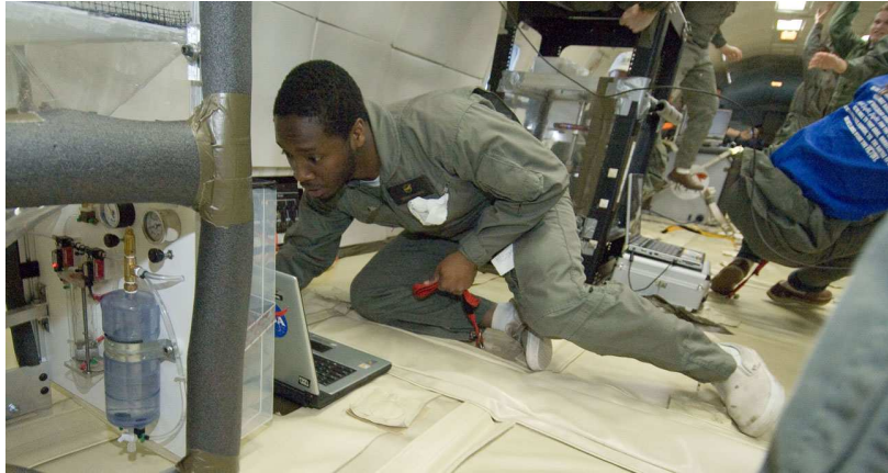
Figure 10. Zero gee pump under test during NASA Microgravity University flight.
