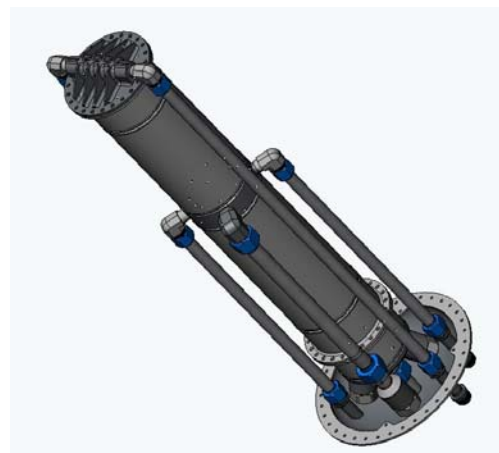
Figure 1. Pistonless pump with stacked cylindrical chambers
