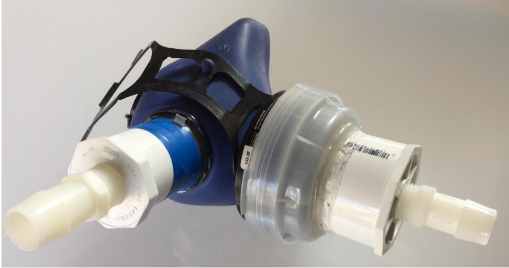
Figure 5: Here is the complete hacked together painting respirator with PVC fittings glued and or taped to the inlet and exhaust. The head gear may need to be reinforced for the extra pressure. The mask may be reinforced so that it doesn't leak along the sides of the nose or under the chine by using a piece of sheet metal, such as a metal binder prong. It can be glued onto a silicone rubber mask with silicone adhesive.
