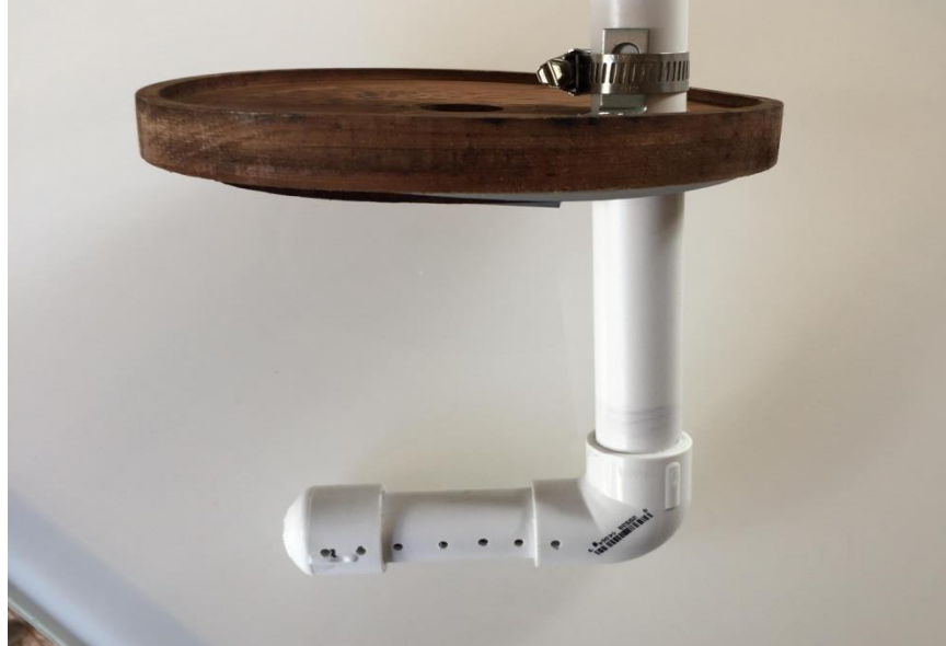
Figure 7: Here is the bubbler, aka back pressure regulator. It uses 1/8" holes to expel exhaled air underwater to provide a back pressure according to the depth. This is placed in a top-vented container. It could also be clamped to the side of a bucket. Adding bleach or dish soap should destroy viruses. Smaller holes lead to smaller bubbles and less chance of the virus making it out of the bucket inside of a large bubble.
