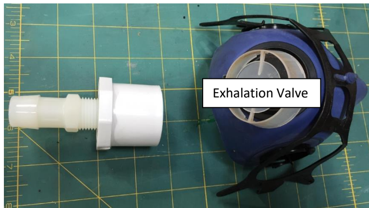
Figure 4: Here is the respirator before taping on the exhalation fitting. The plastic ring on the exhalation valve may need to be glued to the mask, otherwise it may fall off with the extra weight.
